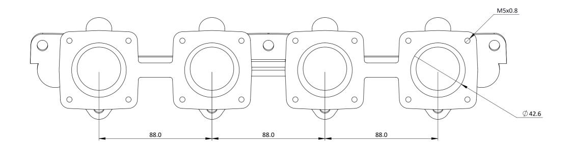
Flanges for Jenvey SF throttle bodies. May be ported out to 46mm at body flange and proportionally at head flange.
