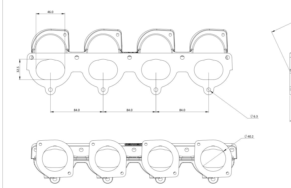
Flanges for Jenvey ST throttle bodies or SF with spindle mods. May be ported out to 45mm at body flange and proportionally at head flange. 2 bosses at ends and 4 on underside for vacuum tappings
