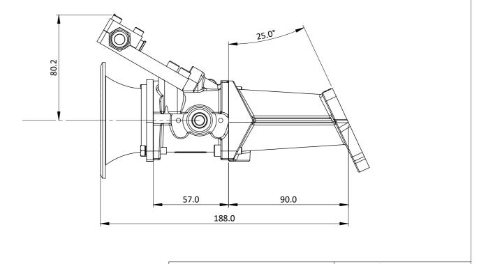
The Jenvey Dynamics tapered CKPG04 kit promises enhanced performance and better throttle control for the TU5JP4 & TU5JP4s engine as found in the VTS, VTR & GT models. This kit contains, an inlet manifold, four ST45 tapered throttle bodies (42mm butterfly), fuel rail, fuel rail mounts and 40mm long airhorns.
