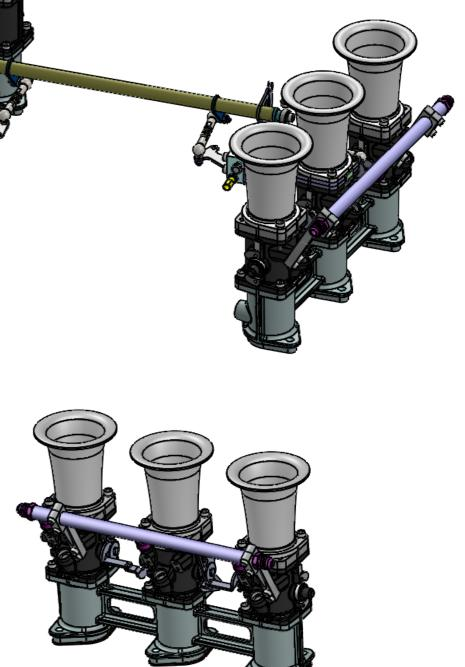
The Porsche 2 stud small bore ITB throttle body kit includes six SF45 taper throttle bodies with a special balanced linkage, two inlet manifolds, heat insulating spacers, fuel rails and six 90mm long taper airhorns. Jenvey throttle bodies and throttle body accessories are engineered for Motorsport, offering excellent performance, reliability, lightness and value. This kit is for early 911s from the 2.0L to the 3.0L and is ideal for road, track or rally use. Made to order.
