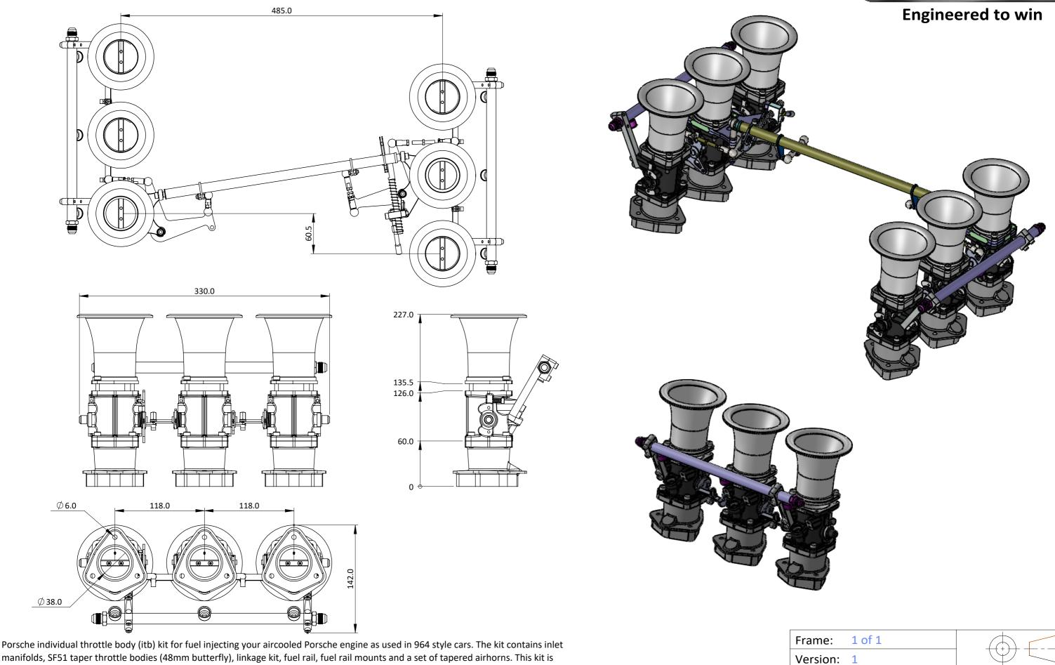
manifolds, SF51 taper throttle bodies (48mm butterfly), linkage kit, fuel rail, fuel rail mounts and a set of tapered airhorns. This kit is for the 3.6 and 3.8 litre 964 cars. Made to order.
